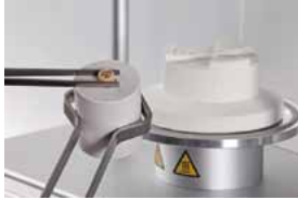
Place the VINTAGE LD Press ingot into the hot investment ring with the shade imprint facing upward.
