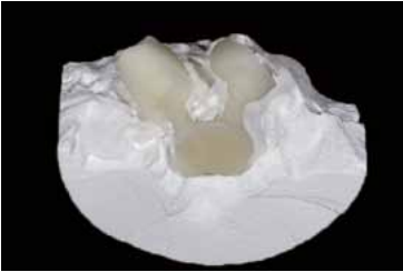
Rough divestment with \text{Al}_2\text{O}_3 at a pressure of approx. 0.2-0.3 MPa (2-3 bar)
