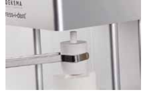
Place the completed investment ring in the center of the preheated press furnace.
