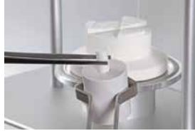
Then place the disposable plunger into the hot investment ring.
