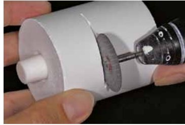
Separate the investment ring by using a separating disk
