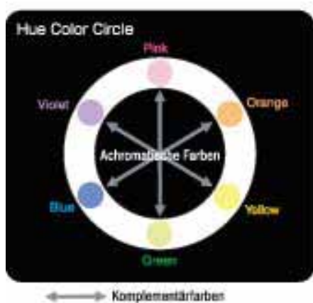
Figure 6 : The color circle shows the primary colours Pink, Yellow and Blue, with the secondary colours arranged in between. The achromatic colours are located at the center of the circle. Colours located opposite each other in this circle are known as complementary colours. If mixed in equal quantities, complementary colours will neutralize each other and turn grey. This phenomenon is based on the subtractive color mixing theory.
