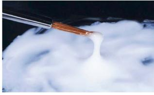
Vintage Art Universal Glazing Powder mixed with conventional mixing liquid, results in a milky mixture, actual shade and translucency is visible only after vacuum firing.
